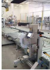
The **gantry palletizer** is a simple and compact system. It can be provided as a stand-alone machine or as an integration to Mad's case packer all in one frame. Like our every other machine it can be interfaced with the Brain 4.0 software by means of a user friendly HMI.
