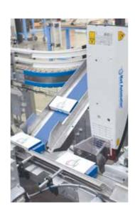
It is available either with laser or ink marking technology both in colors or black and white. The print position is adjustable and settable on multiple lines. The marker can print all the data relevant to the productionlot, such as the production date, the expiration date, the identification number, etc... to grant total product traceability.
