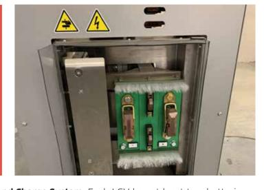
**Fully automatic Change and Charge System**. Each LGV has at least two batteries that are automatically alternated; the LGV moves to the area adjacent to the battery swap and charge station. It automatically delivers the empty battery to the charging station and takes the full battery on board, than it proceeds to complete its tasks. This system can be combined with any type of battery.
