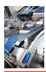
The Weight Control System is an essential tool to guarantee the quality of the final package and to ensure the respect of the correct product quantity in the case. It is a high-performance device, integrated into the system, which suitable for a wide range of weights and sizes. It can also control the cases' loading and the non conforming product rejectionbefore they reach the marking and loading stations.
