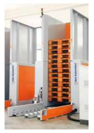
tStacker is designed to handle empty pallet stacks. It is an easyto-use system; thanks to the touch screen panel, the operator can independently configure the number of pallets to be stacked/unstacked.
