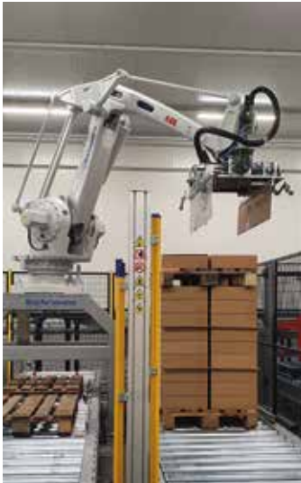
Robotic palletizer features a gripper head.
